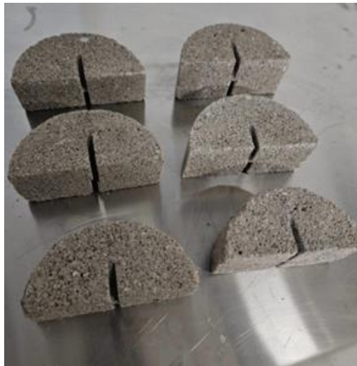
Fig.3 Prepared SCB specimens with notch cracks
