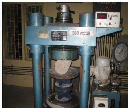
Split Tensile Test on Pervious Concrete Cylinders
