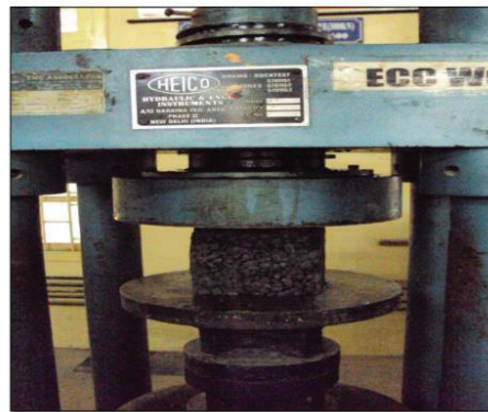
Fig. 4.1 Compression Test on Pervious Concrete Cubes
