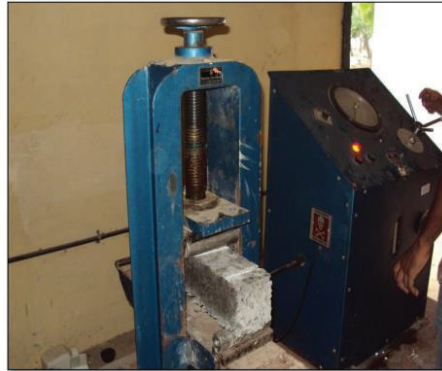
Flexural test on pervious concrete prism
