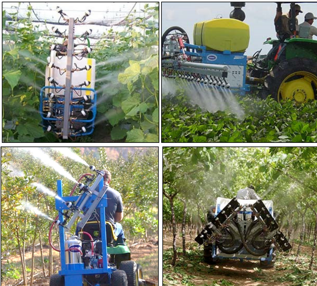
Figure 2. Some pesticide electrostatic sprayers that were developed by ESS company using MaxCharge nozzles ( https://maxcharge.com/ ).
