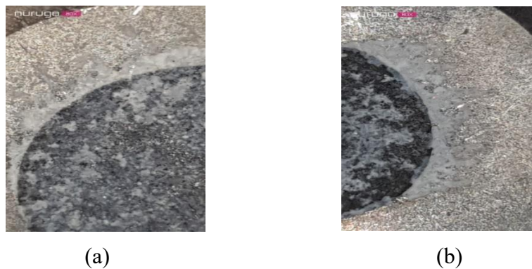
Figure 3. Potentiodynamic polarization test corrosion images of (a) Al7075/AS21 and (b) Al7075/Mg2Zn bimetal composites.
