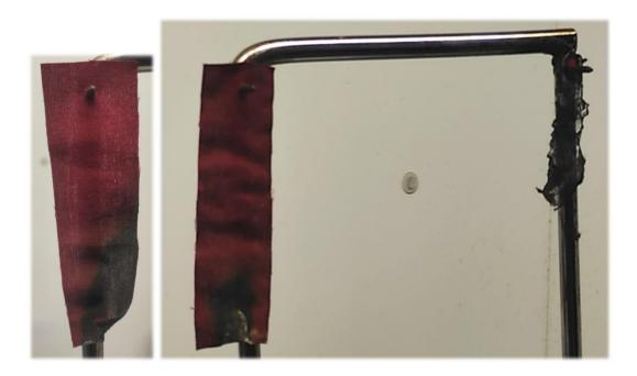
Figure 4: Sequentially, the appearance of fabric samples treated with AP-1 polymer solution, fabric samples treated with AP-1 polymer solution and subjected to washing, and fabric samples treated with water only and dried after the burning test.
