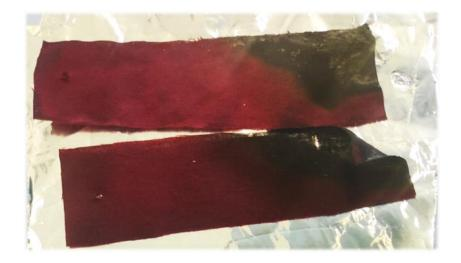
**Figure 5:** Appearance of fabric samples after vertical burning test conducted following treatment with AP-1 polymer solution.
