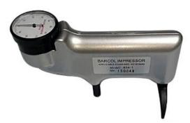
Figure 4. Barcol hardness tester
